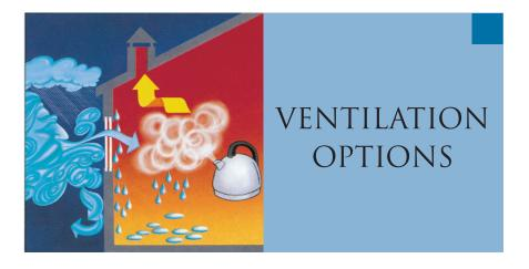
After reducing moisture sources, ventilation may be used to improve indoor air quality. All ventilation systems should be balanced—the amount of air in equals the amount of air out—with intakes sized to allow easy entry of enough air to supply all exhaust devices.
