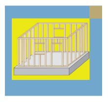
for mold, is to avoid building basements at all. Frost-protected shallow foundations are a good alternative. (Details are available in training materials from CMHC's Assisted Housing Division, particularly the Building Technical Excellence workshop developed through cooperation between CMHC and the Ontario First Nations Technical Services Corporation.)
